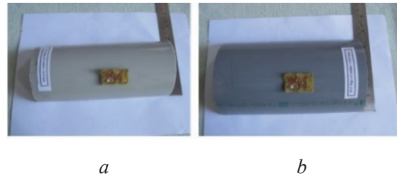
Figure 9 – Picture of the suggested antenna curved around internal radii: ( a – 54.5 mm; b – 44.5 mm) PVC pipes [58]
