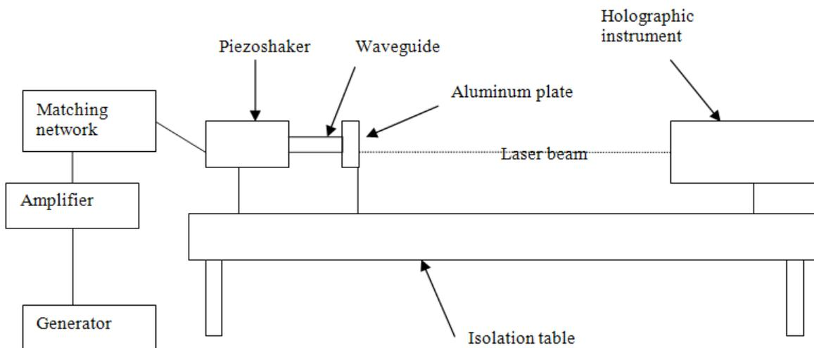
Figure 3 – The scheme for the measurement of vibrations of waveguide by holographic interferometry
