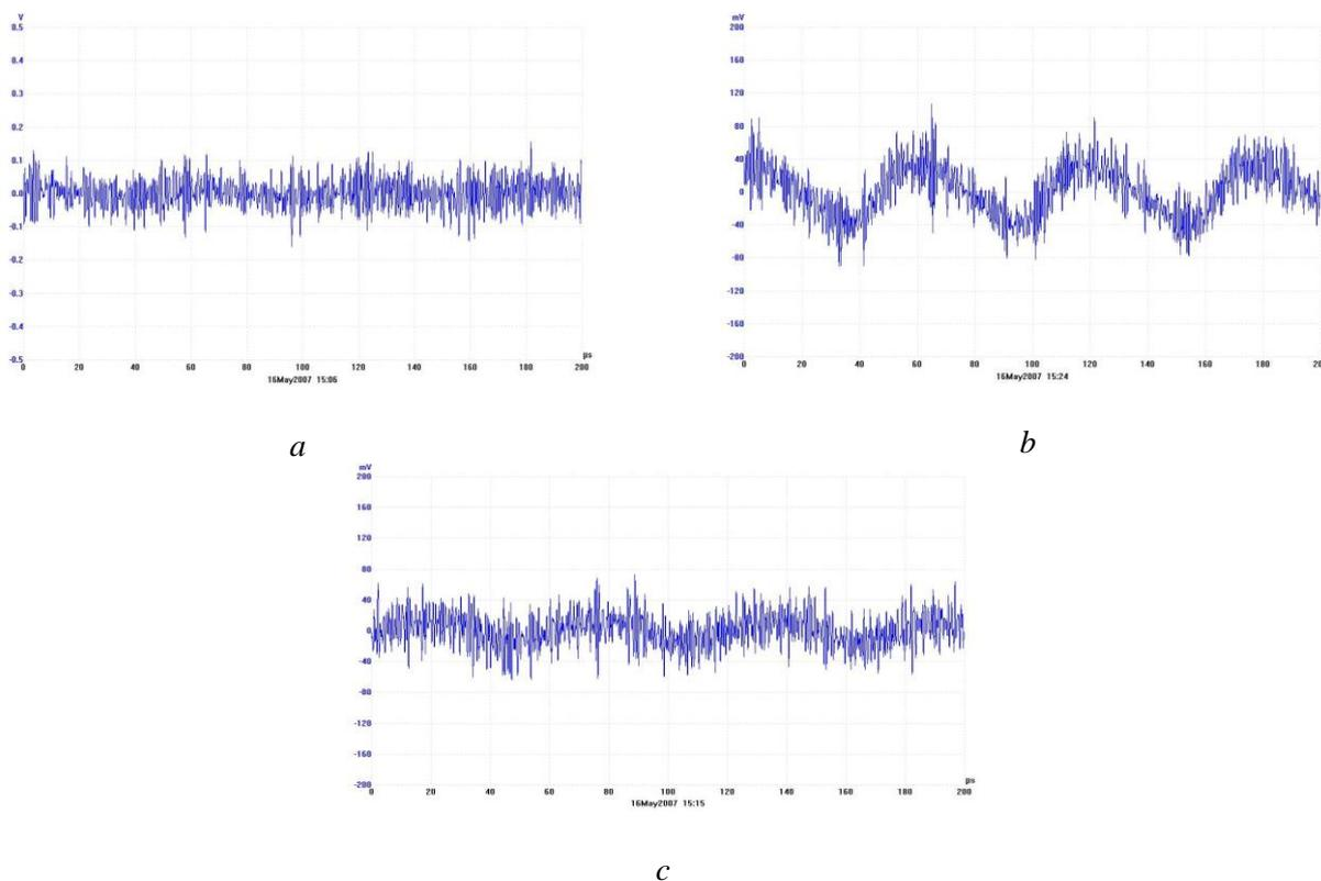
Figure 4 – Results of the same frequency (17 kHz), but different amplitudes: a – 100 mV; b – 400 mV; c – 600 mV
