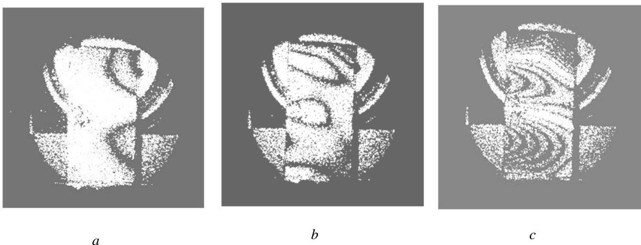
Figure 5 – The holographic interferograms of the same amplitude (100 mV), but different frequencies:  $a$  – 12 kHz;  $b$  – 17 kHz;  $c$  – 19 kHz
