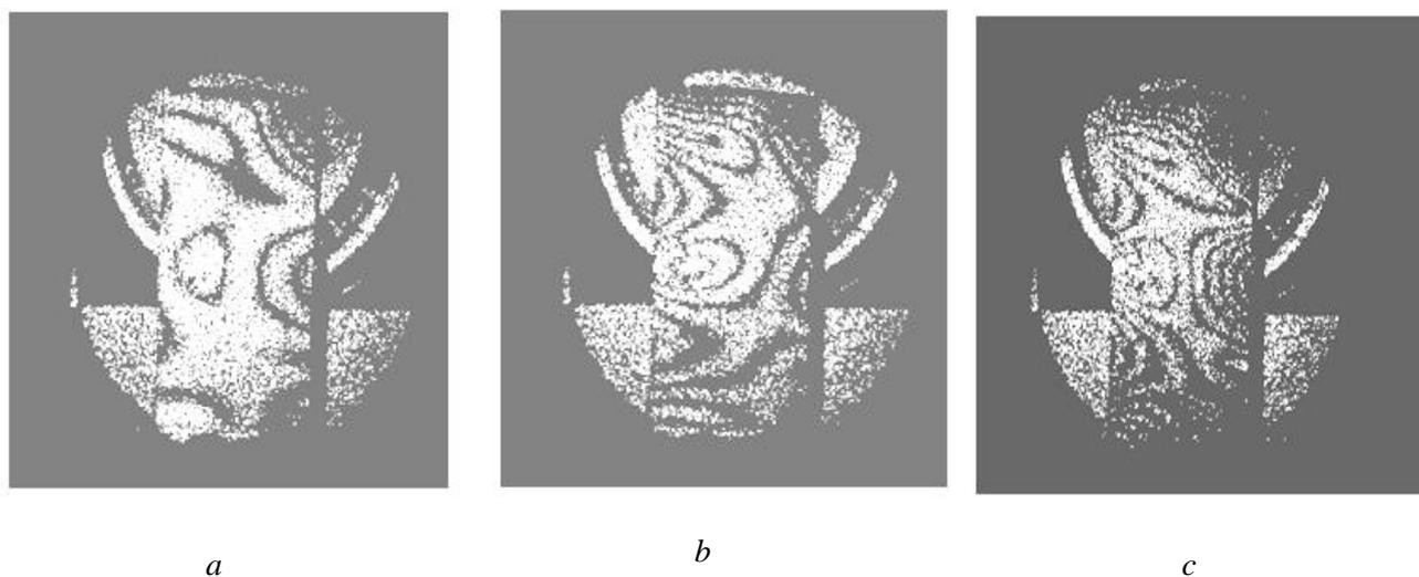
Figure 6 – The holographic interferograms of the same frequency (17 kHz), but different amplitudes:  $a$  – 150 mV;  $b$  – 300 mV;  $c$  – 600 mV
