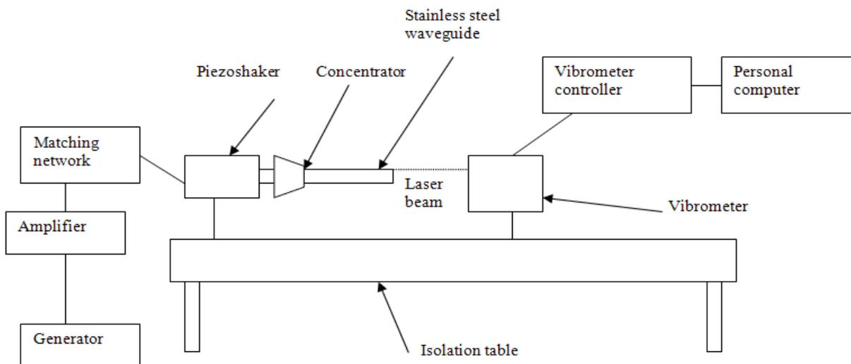
Figure 2 – The scheme for the measurement of vibrations of waveguide by vibrometer
