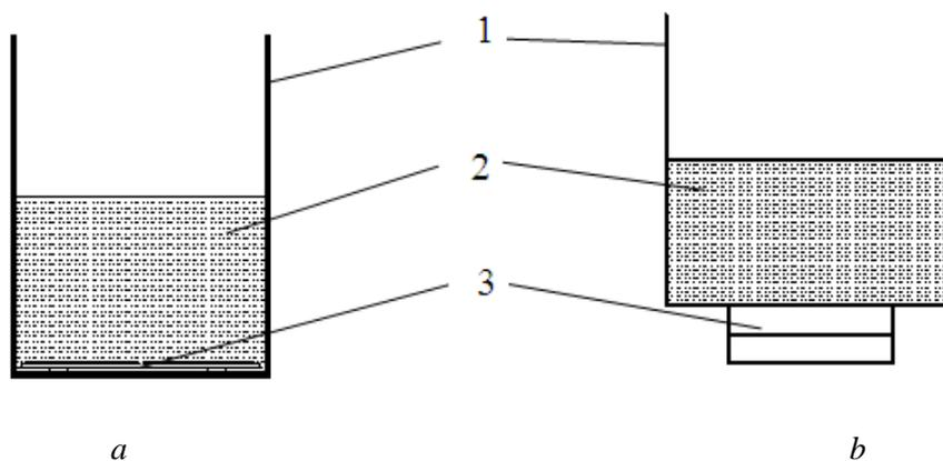
Figure 1 – MRF mixer with piezoelectric element: *a* – piezoelectric element is attached to the bottom of the vessel inside and immersed into the MRF; *b* – piezoelectric element is attached to the bottom of the vessel outside; 1 – metal vessel, 2 – MRF, 3 – piezoelectric element
