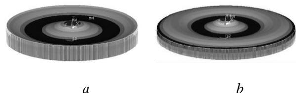
Figure 5 – rotational symmetric normal modes: a – 3<sup>rd</sup> with 2012 Hz; b – 4<sup>th</sup> with 4430 Hz
