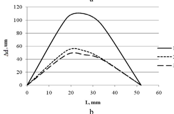
Figure 4 – Displacements of elastic carbon fiber plates with different voltages (1 – 10 V; 2 – 30 V; 3 – 50 V): a – plate length  $L = 44 \text{ mm}$ ; b – plate length  $L = 52 \text{ mm}$
