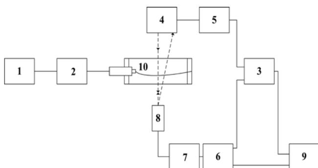
Figure 2 – Experimental set up: 1 – signal generator Agilent 33220A; 2 – power amplifier EPA-104; 3 – analog digital converter (ADC) «PicoScope-3424»; 4 – laser displacement sensor LK-G82; 5 – laser sensor controller LK-G3001PV; 6 – Polytec OFV-5000 vibrometer controller; 7 – Polytec OFV-512 fiber interferometer; 8 – Polytec OFV-130-3 micro-spot sensor head; 9 – computer; 10 – piezoelectric laser beam shutter
