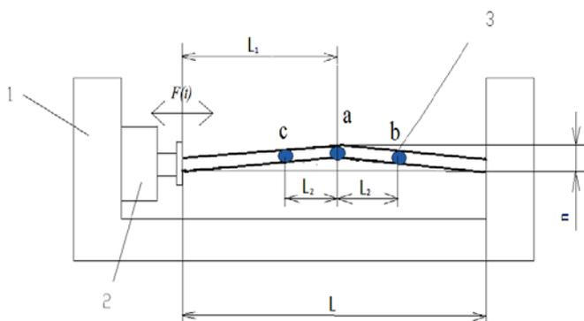
Figure 3 – The scheme of experimental measurements:  $a, b, c$  – the points where measurements of displacements of carbon fiber plate were made;  $n$  – primary deflection of the carbon fiber element
