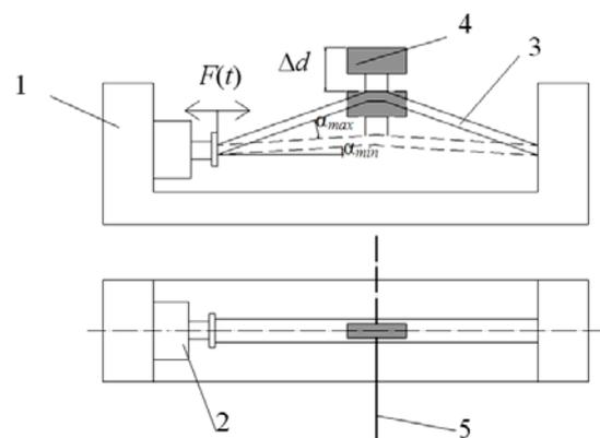
Figure 1 – Scheme of the developed piezoelectric laser shutting system: 1 – housing; 2 – multilayer piezoelectric actuator; 3 – carbon fiber element; 4 – laser beam covering plate; 5 – laser beam
