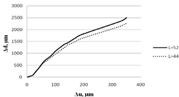
Figure 5 – Dependence of displacements  $\Delta d$  of point  $a$  of the elastic carbon fiber plate on piezoelectric actuator displacements  $\Delta u$  for the plate lengths  $44 \text{ mm}$  and  $52 \text{ mm}$
